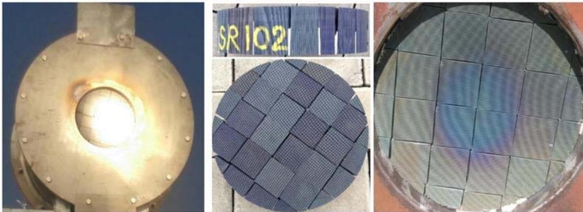
Figure 10 - Volumetric absorber material. (left) During testing; (center) before (right) after 20h
