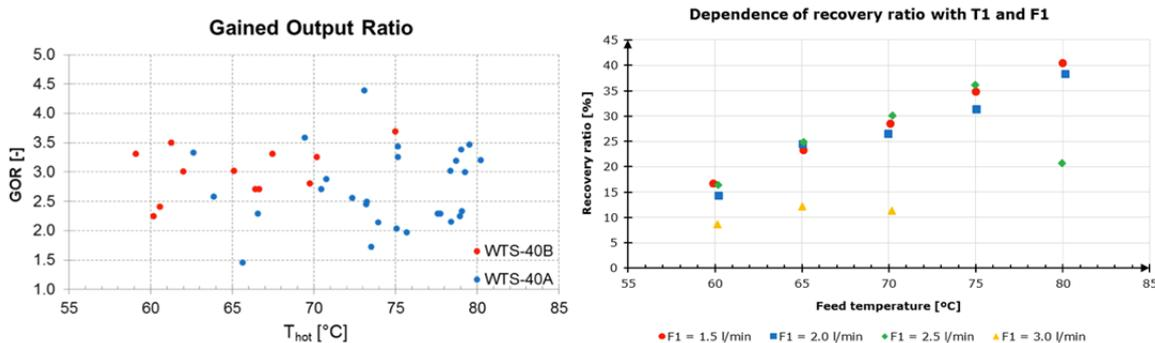
Figure 3 - Gain Output Ratio (left) and Recovery Ratio (right) vs hot inlet temperature and flow for ME-VA MD modules
