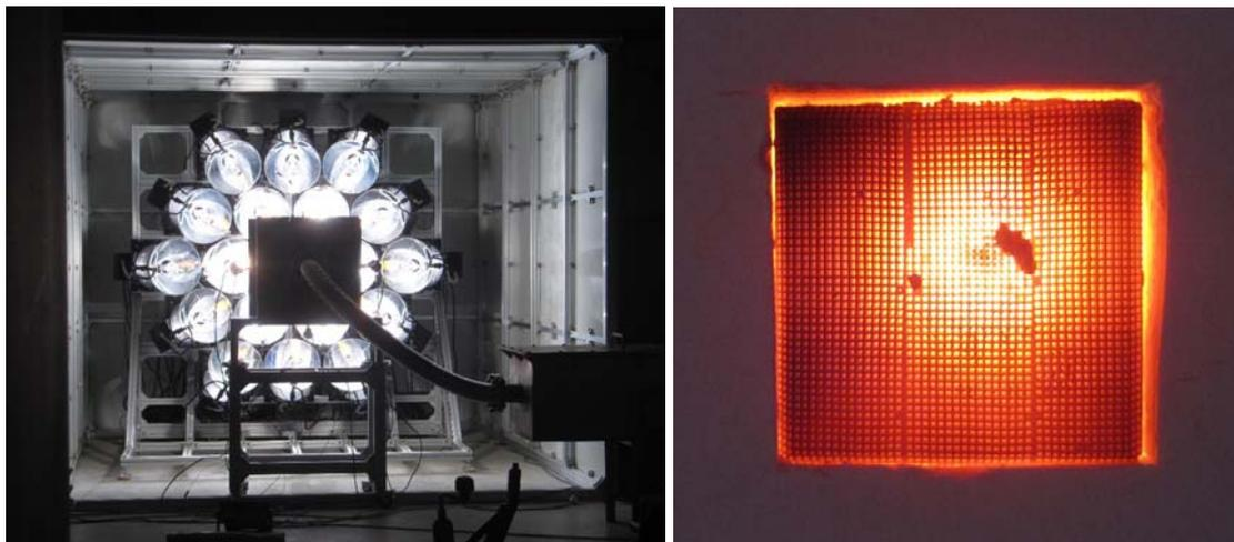
Figure 11 - Left, photograph of the IEECAS new 30 kW<sub>th</sub> high flux solar simulator during operation. Right, siliconized silicon carbide monolithic honeycomb photographed immediately after ceasing operation of the solar simulator, at temperatures in excess of 1300 °C
