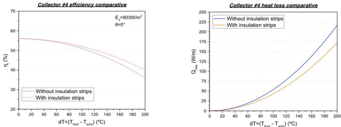
Figure 2 - Efficiency and heat loss comparative using the insulation strips proposed by KSU
