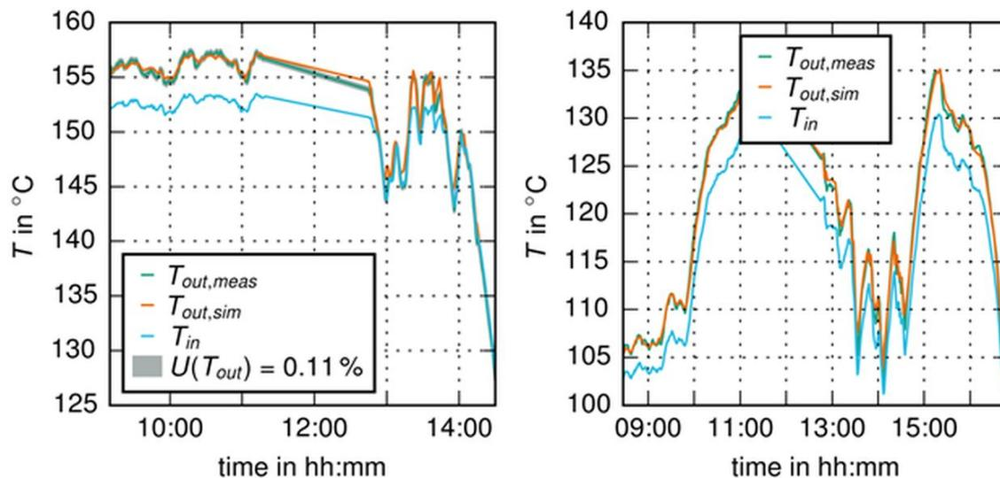
Figure 9 - Example evaluation of dynamic testing - comparison of simulation using identified parameters and measurements
