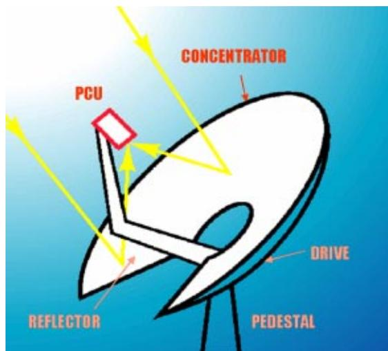
Fig. 1 Dish Stirling system components
