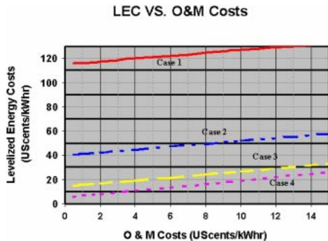
**Fig. 19 Levelized energy cost versus O&M costs**
