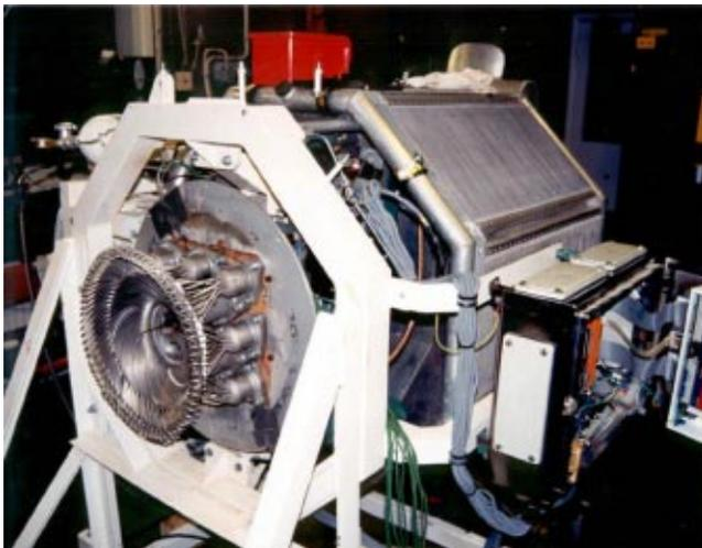
Fig. 11 Kockums 4-95 kinematic Stirling engine
