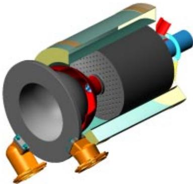
Fig. 17 BioDish hybrid receiver
