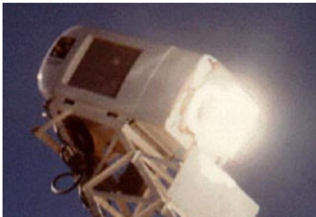
Fig. 3 STM Power engine during on-sun operation
