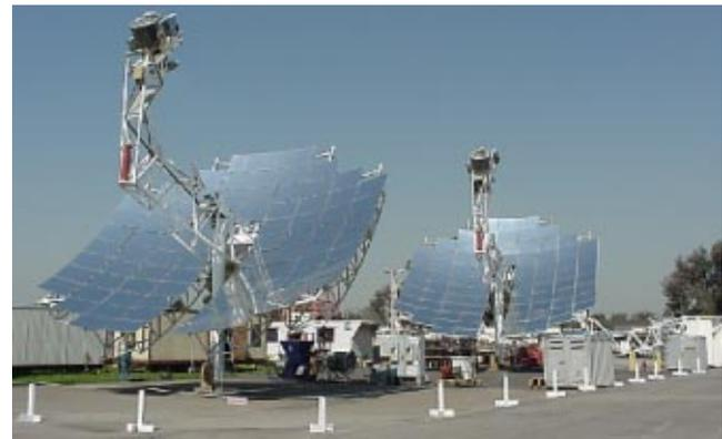
Fig. 10 SES systems on test at Huntington Beach, California
