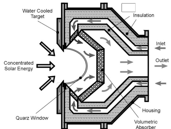
Fig. 18 DLR pressurized volumetric air receiver
