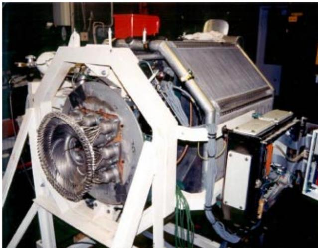
Fig. 11 Kockums 4-95 kinematic Stirling engine
