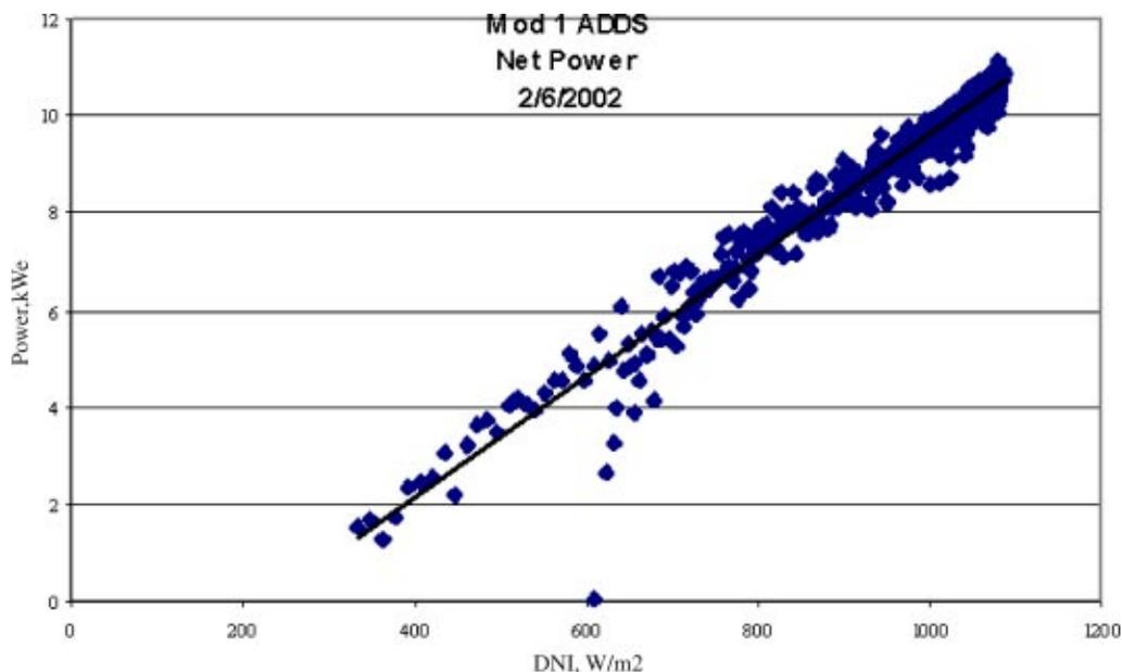
Fig. 16 Mod 1 ADD system net power output versus direct normal insolation
