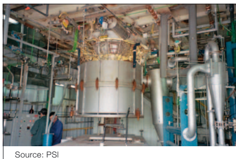
Figure 18: 300 kW th solar chemical pilot plant developed and tested in the EU's R&D project SOLZINC – The two-cavity reactor (1.4 m inner diameter) for the carbothermal reduction of ZnO is specifically designed for beam-down incident radiation, as obtained at the solar tower research facility at WIS, Israel.
